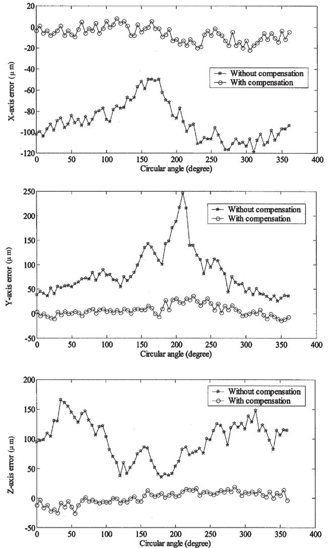
Fig. 6. Results of error compensation for path S.
