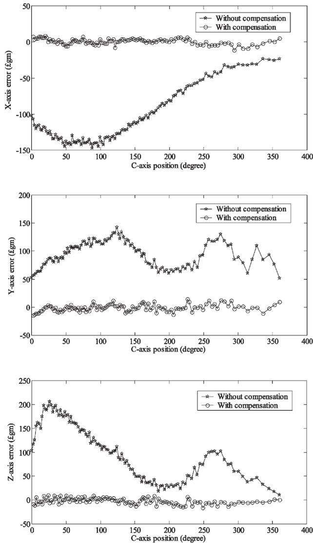
Fig. 5. Results of error compensation for path F.
