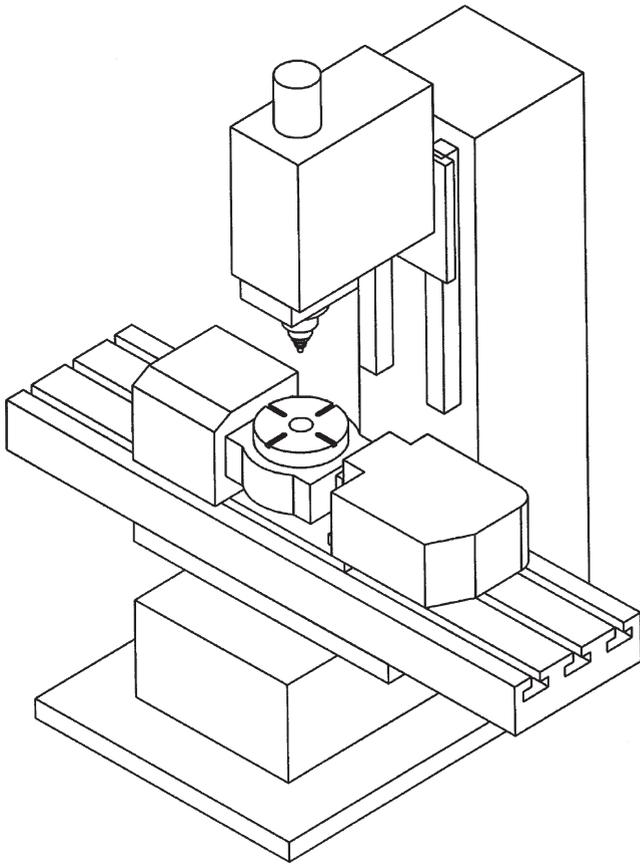
Fig. 1. Five-axis milling machine of the type  $X'Y'ZA'C'$ .
