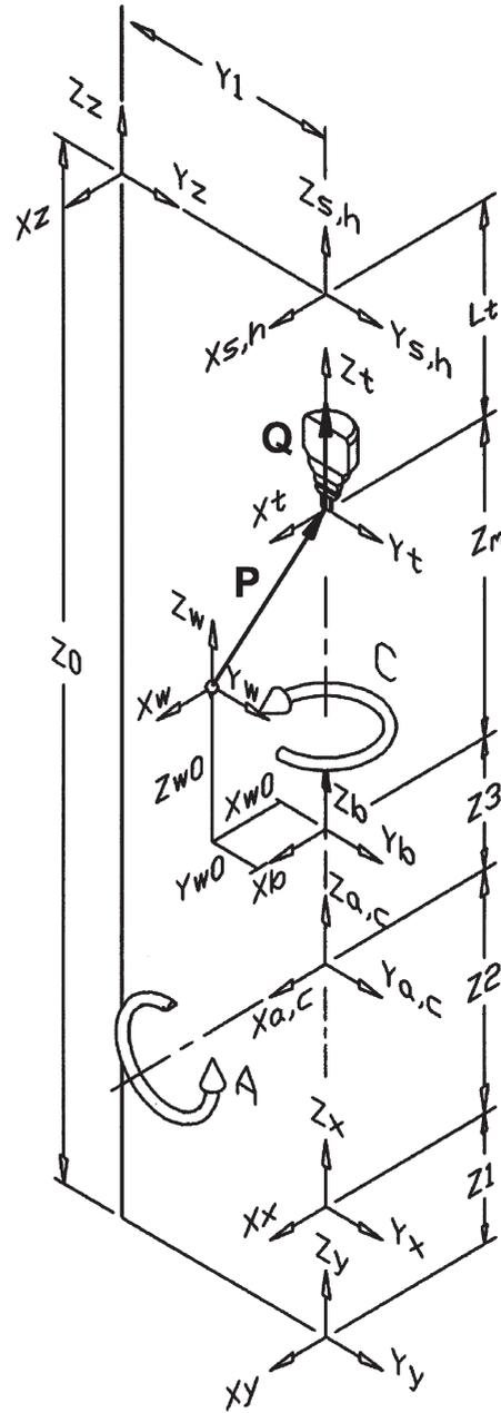
Fig. 2. The coordinate frames of the five-axis milling machine.
