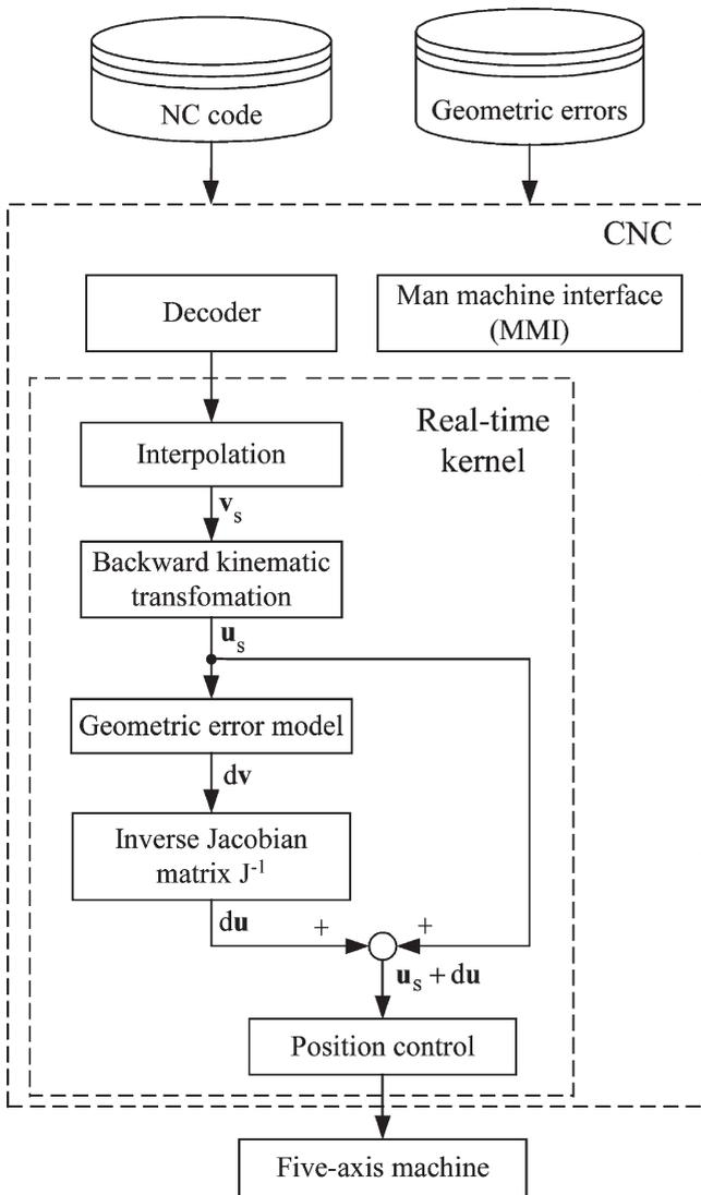
Fig. 3. The functional structure of real-time geometric error compensation.
