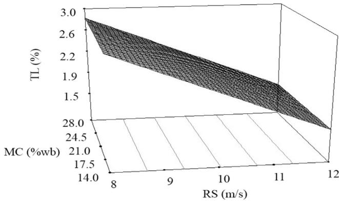
Fig. 3. Response surface plot of shelling unit loss (TL) showing the effect of moisture content (MC, measured on a weight basis, %wb) and rotor speed (RS), when feed rate was 1.5 t/hr.
