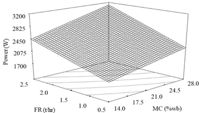
**Fig. 6.** Response surface plot of power consumption (P) showing the effect of feed rate (FR) and moisture content (MC, measured on a weight basis, %wb), when rotor speed (RS) was 10 m/s.
