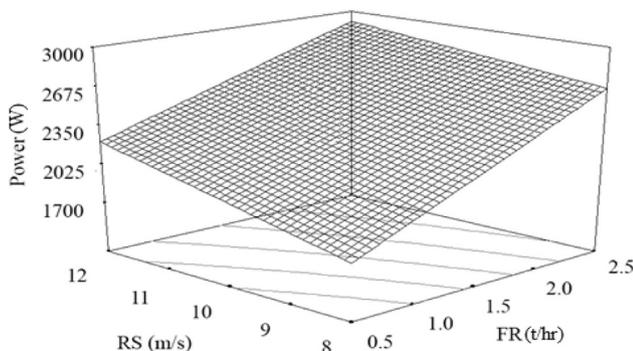
**Fig. 8.** Response surface plot of power consumption (P) showing the effect of feed rate (FR) and rotor speed (RS), when moisture content was 14% on a wet basis.
