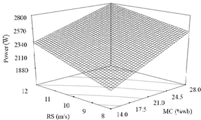
**Fig. 7.** Response surface plot of power consumption (P) showing the effect of moisture content (MC, measured on a weight basis, %wb) and rotor speed (RS), when feed rate was 1.5 t/hr.
