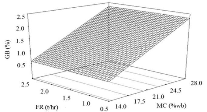
Fig. 5. Response surface plot of grain breakage (GB) showing the effect of feed rate (FR) and moisture content (MC, measured on a weight basis, %wb), when rotor speed was 10 m/s.
