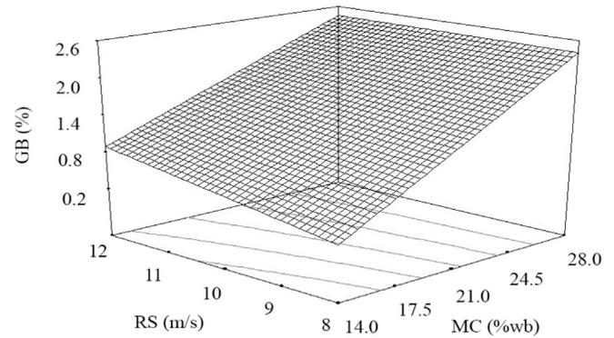
Fig. 4. Response surface plot of grain breakage (GB) showing the effect of moisture content (MC, measured on a weight basis, %wb) and rotor speed (RS), when feed rate was 1.5 t/hr.
