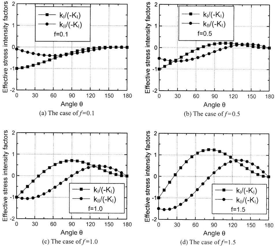
Fig. 2. Variation of effective stress intensity factors  $k_I$ ,  $k_{II}$  with angle  $\theta$ , for different  $f$ .
