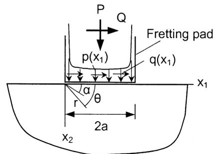
Fig. 1. Contact between a two-dimensional rectangular punch and a substrate.
