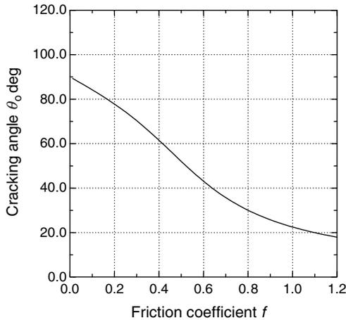
Fig. 3. Cracking angle  $\theta_0$  versus friction coefficient  $f$ .
