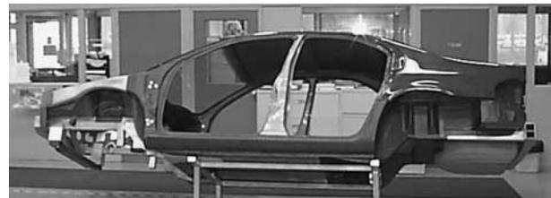
Fig. 1. Carbon fiber body.
