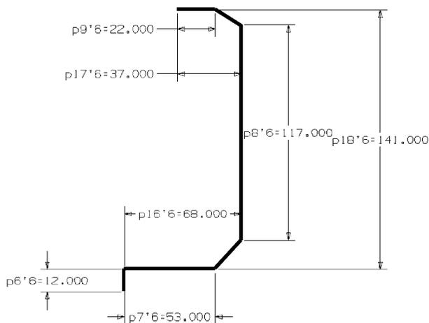
Fig. 2. Outer piece of upper rail.
