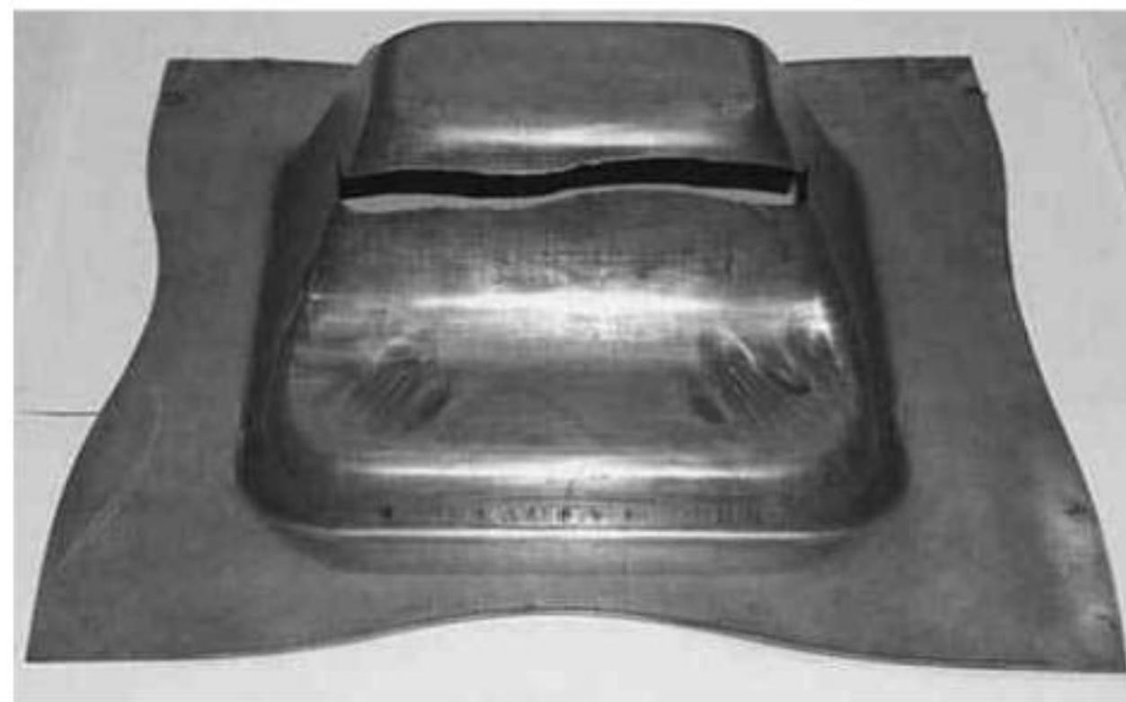
Fig. 7. Split and wrinkles in the production part.
