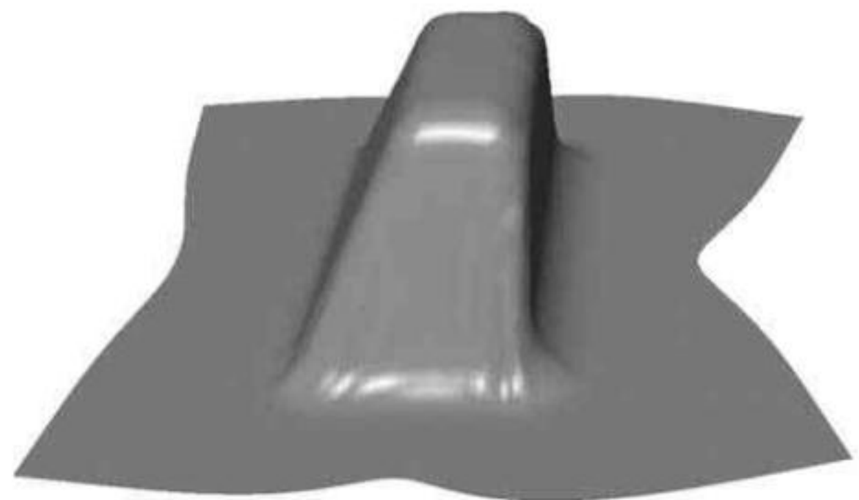
Fig. 12. Simulated shape for the modified die design.
