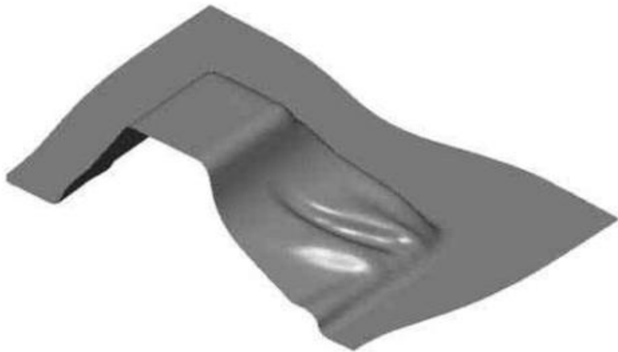
Fig. 10. Wrinkle formed when the sheet blank touches the stepped edge.
