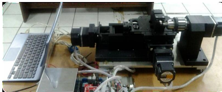
Figure 6. CNC Lathe Machine complete technical prototype
