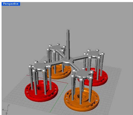
Fig. 4. The configuration of sprue, runner and gate.
