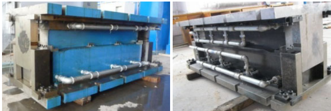
Fig. 5 Hot stamping die with different design of cooling system
