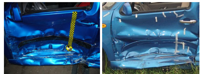
Fig. 13 Vehicle side impact contrast of cold bending pipe (left) and hot forming door beam (right)
