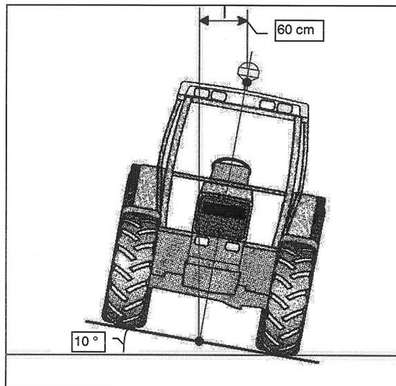
Fig. 1. Difference in position for two locations due to sloping terrain.
