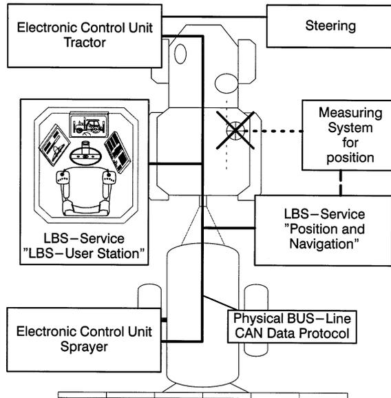
Fig. 2. Scheme of an agricultural network in a tractor-sprayer combination.
