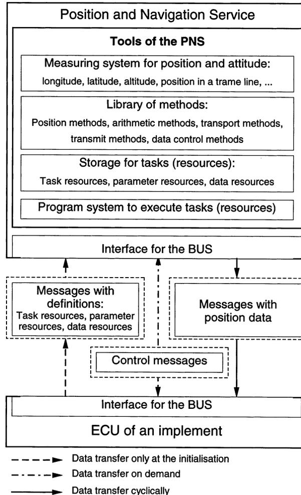
Fig. 3. Structure of a PNS and its data exchange with one ECU.
