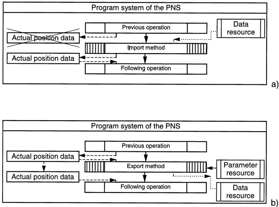
Fig. 6. Examples of the use of transport methods in the course of a task resource. (a) Import method; (b) export method.
