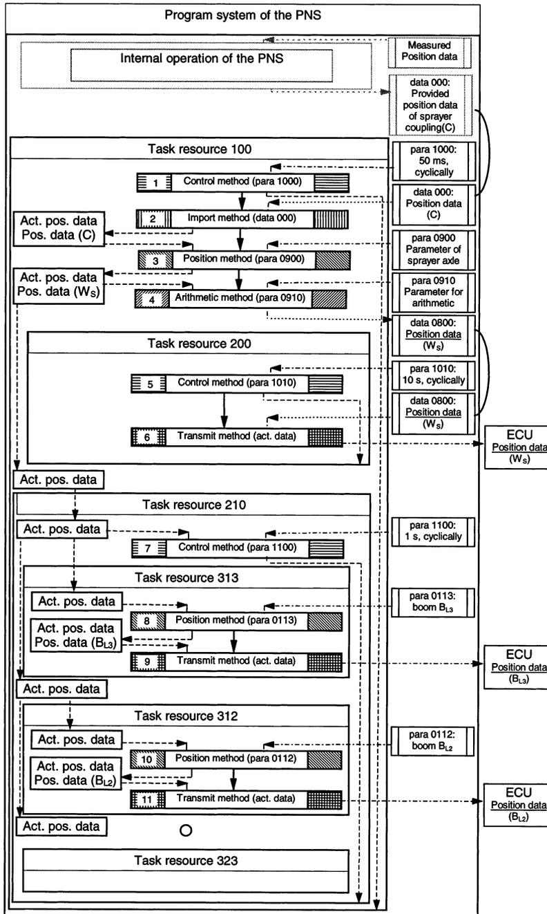
Fig. 9. Structure of an exemplary task resource for the sprayer.
