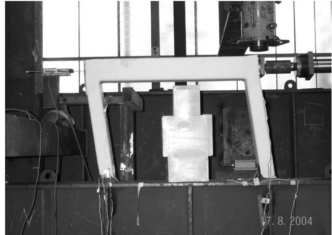
Fig. 2. Lateral load testing of K275 ROPS.
