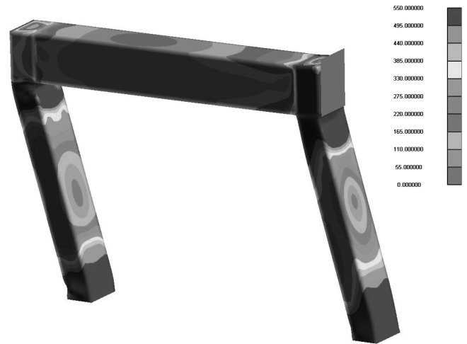
Fig. 9. Von Mises stress distribution and plastic hinges during impact.
