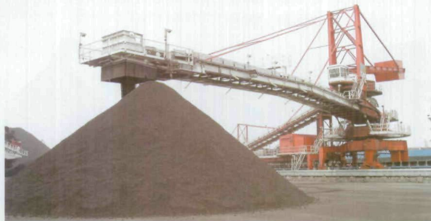
The Sandvik PS100 luffable and sleuable stacker is used in standard, heavy duty applications.
