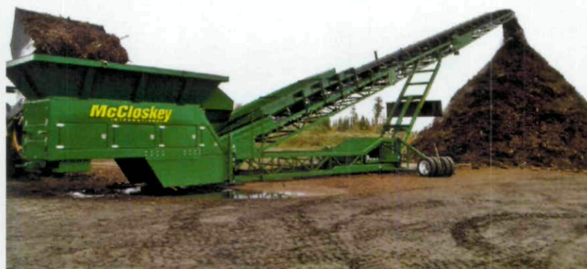
McCloskey feeder stackers are used in wood waste, bark, compost, and topsoil applications.
