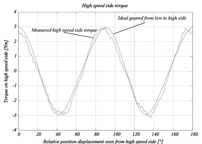
Fig. 6. Measured and ideal geared torque on high-speed side.
