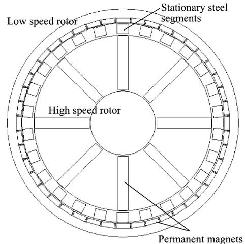
Fig. 1. Cross section of the considered magnetic gear.
