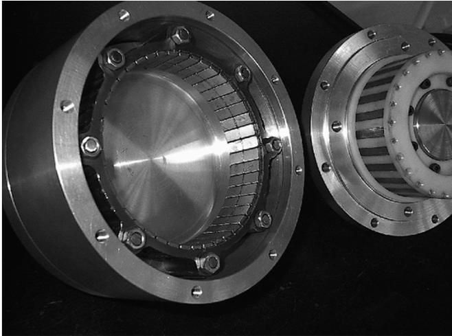
Fig. 4. Photograph of the constructed gear.
