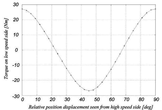
Fig. 3. Torque on low-speed side versus relative position displacement on the high-speed rotor side.
