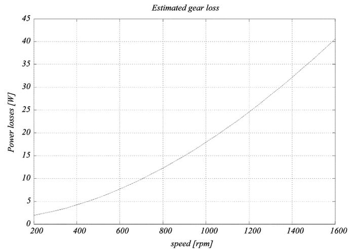
Fig. 9. Estimated magnetic gear losses without "magnetic" bearing losses.
