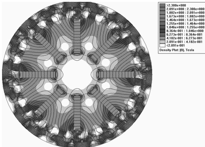
Fig. 2. Calculated flux lines and induction for magnetic gear.
