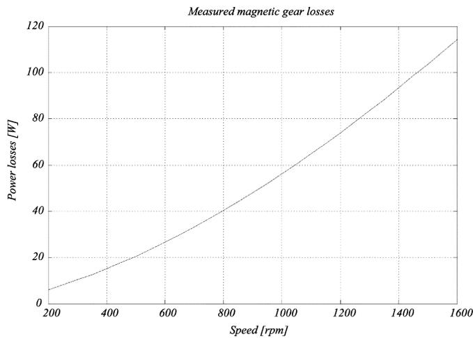
Fig. 7. Measured magnetic gear losses.
