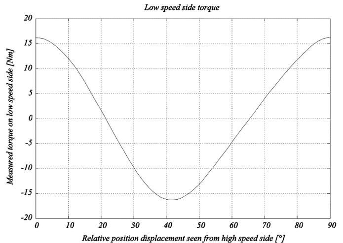
Fig. 5. Measured torque on low-speed side.
