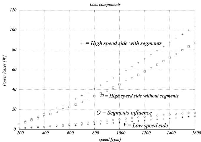
Fig. 8. Extraction of different loss components in the magnetic gear.
