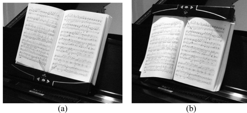
Fig. 7. PageFlip Lite clipped to (a) bottom and (b) top of book. No support stand is needed on piano.
