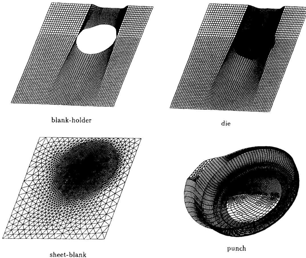
Fig. 8. Mesh system for the original die design.
