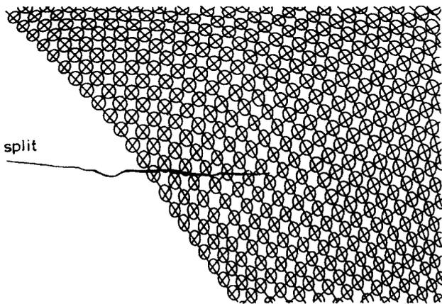
Fig. 6. Deformed circles on the sheet-blank.
