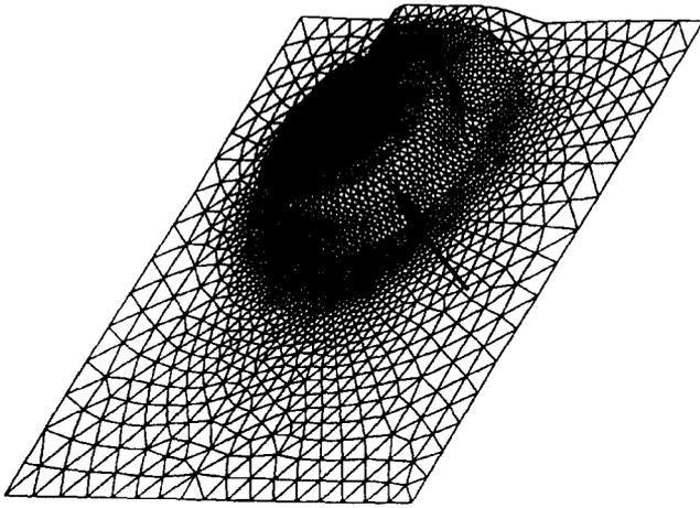
Fig. 9. Deformed shape for the original die design.
