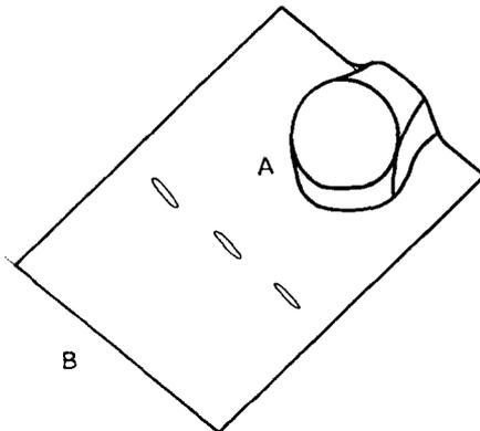
Fig. 3. The location of the drawn cup in the sheet-blank.
