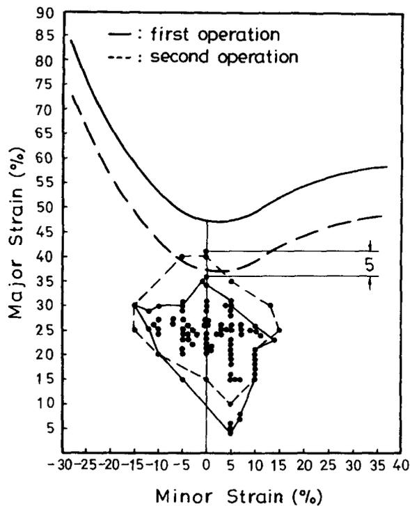
Fig. 17. Measured strains for the first- and second-draws of the optimum die design.
