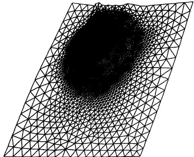
Fig. 14. The deformed shape for the modified die design.
