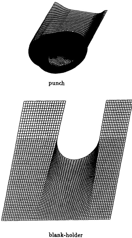
Fig. 12. The modified die design.
