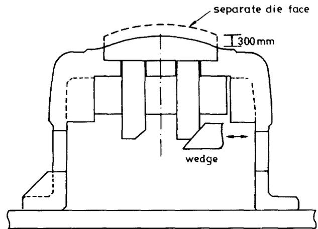
Fig. 15. The separate die face and the wedge mechanism.
