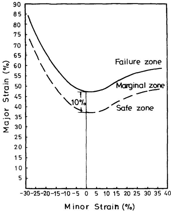
Fig. 5. The forming-limit diagram for 0.7 mm DDQ steel sheet.
