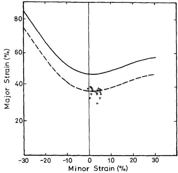
Fig. 13. The strain distribution for the modified die design.
