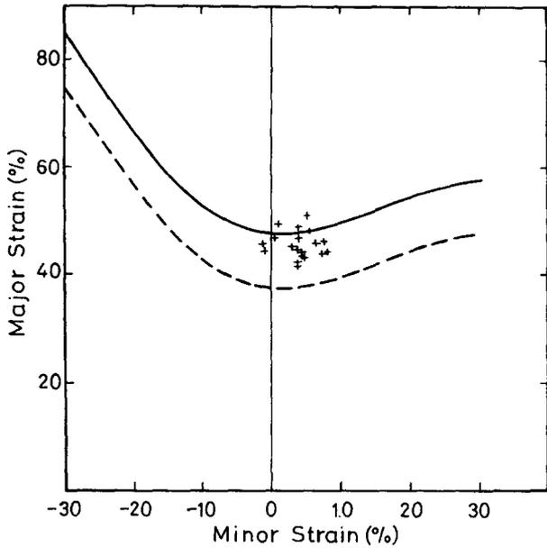
Fig. 11. The strain distribution obtained from finite-element simulation for the original die design.
