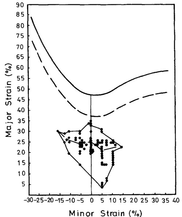
Fig. 16. Measured strains for the first draw of the optimum die design.
