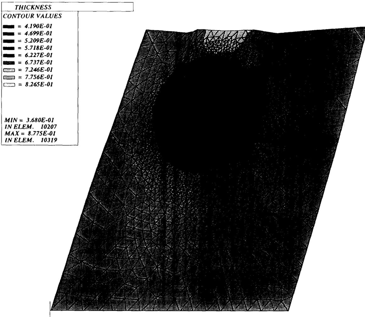
Fig. 10. Thickness contour obtained from finite-element simulation for the original die design.
