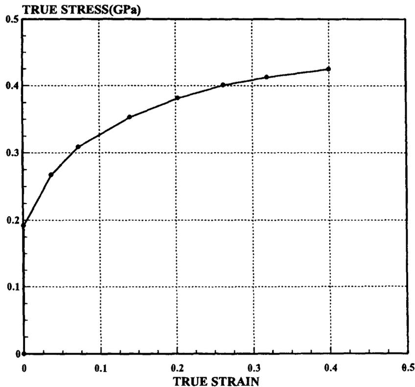
Fig. 4. The stress-strain curve for the sheet-blank.
