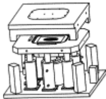
Fig. 2. Blank holder force control system and tooling being developed at the ERC/NSM labs.
