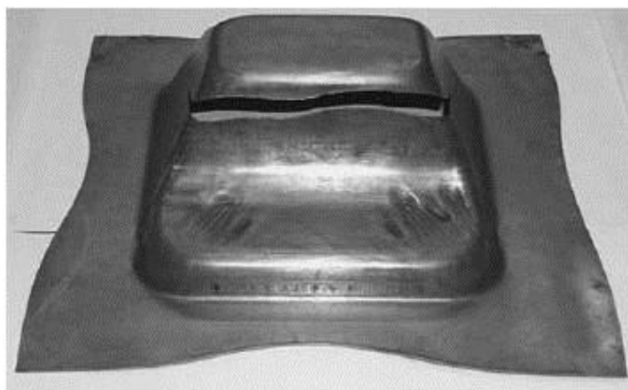
Fig. 7. Split and wrinkles in the production part.
