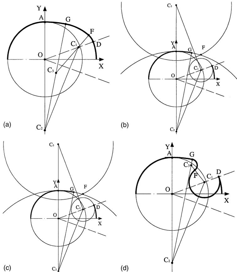
Fig. 3. Examples 1 and 2: graphical representation of design solutions for Eq. (16) and design solutions for Eqs. (16)–(18). Only case (a) is a practical feasible design.
