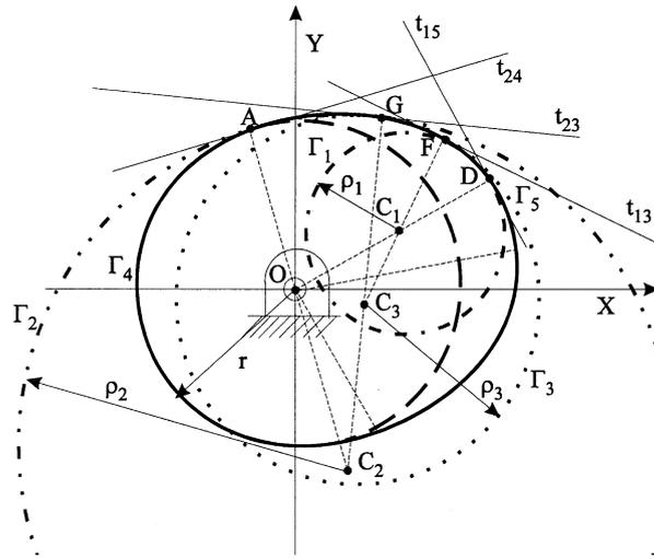
Fig. 2. Characteristic loci for three circular-arc cams.
