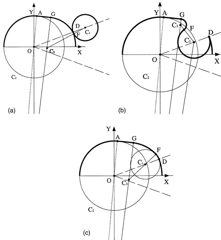
Fig. 5. Example 4: graphical representation of design solutions for Eqs. (16)–(21). Only case (c) is a practical feasible design.
