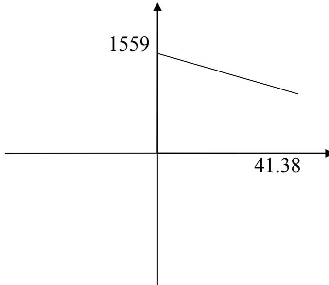
$$\begin{aligned} \textcircled{2} \quad n &= U/K_e \phi - (R_a + R_{ad})T / K_e K_t \phi^2 \\ &= U/K_e \phi - (R_a + R_{ad})T / 9.55 K_e^2 \phi^2 \end{aligned}$$
