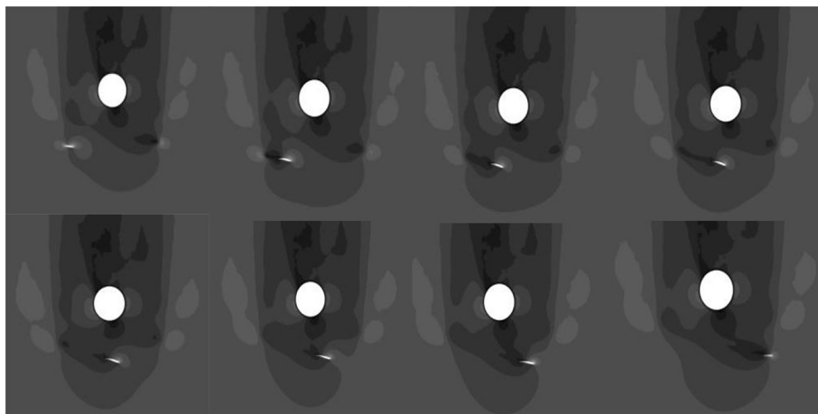
Fig. 11. Velocity contours for L 1 upstream clearance at increasing timesteps.
