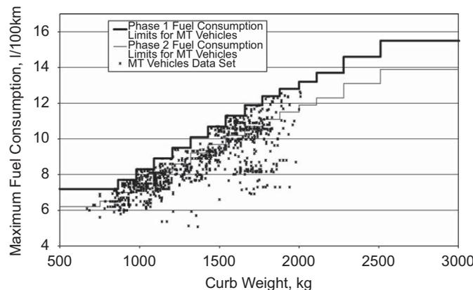
**Fig. 9.** NDRC fuel consumption and weight data for manual transmission passenger cars for sale in China.
