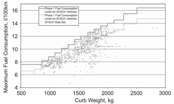
**Fig. 10.** NDRC fuel consumption and weight data for automatic transmission and SUV passenger cars for sale in China.
