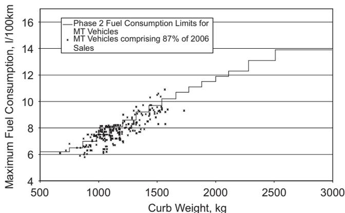
**Fig. 11.** Fuel consumption and weight data for manual transmission passenger cars comprising 87% of car sales in China.
