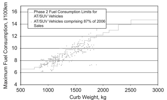
**Fig. 12.** Fuel consumption and weight data for automatic transmission and SUV passenger cars comprising 87% of car sales in China.
