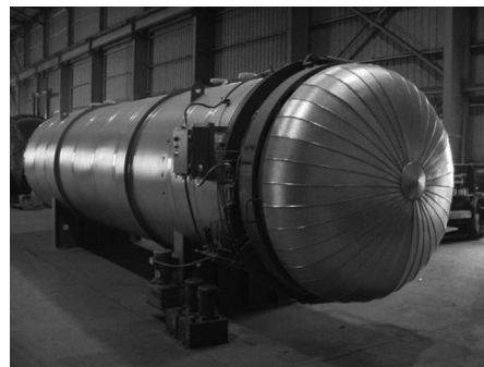
Figure 8.1 A custom built large size autoclave for vulcanizing rubber lined tanks.
