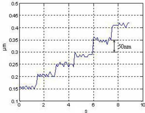
Figure 7: Distance resolution curve of feed mechanism
