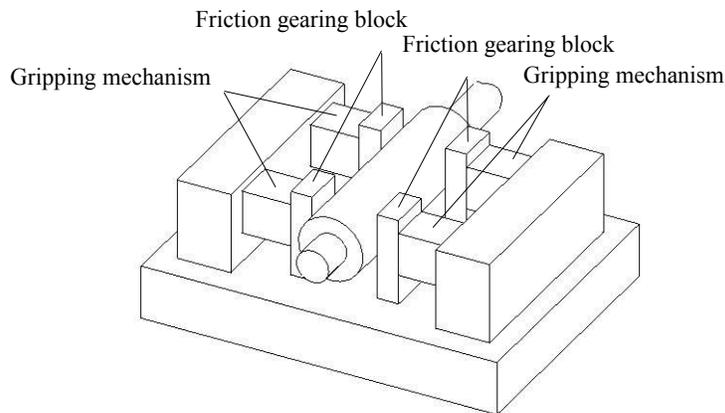
Figure 2: Operating principle of the feeding mechanism
