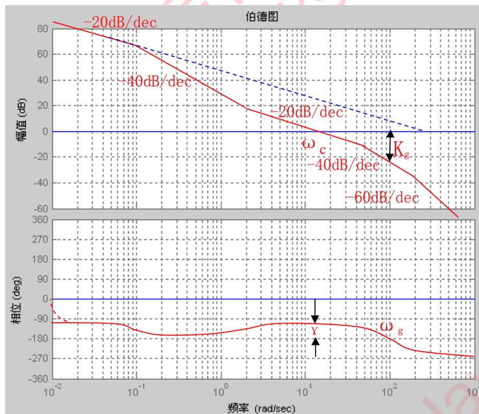
$$\phi(\omega_g) = -90^\circ - \arctan 10\omega_g + \arctan \frac{\omega_g}{2} - \arctan \frac{\omega_g}{50} - \arctan \frac{\omega_g}{200} = -180^\circ$$
