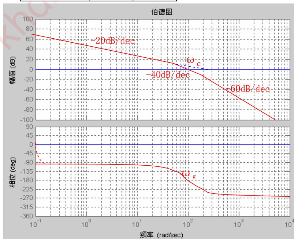
$$\phi(\omega_g) = -90^\circ - \arctan \frac{\omega_g}{50} - \arctan \frac{\omega_g}{200} = -180^\circ$$
