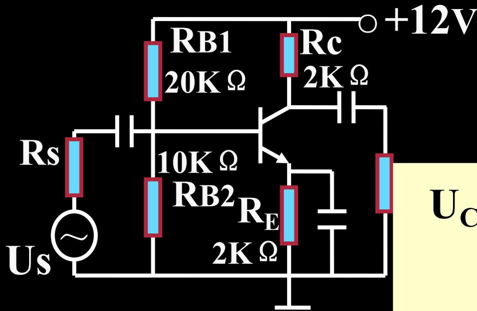
$$U_B = \frac{R_{B2}}{R_{B1} + R_{B2}} \cdot U_{CC}$$
