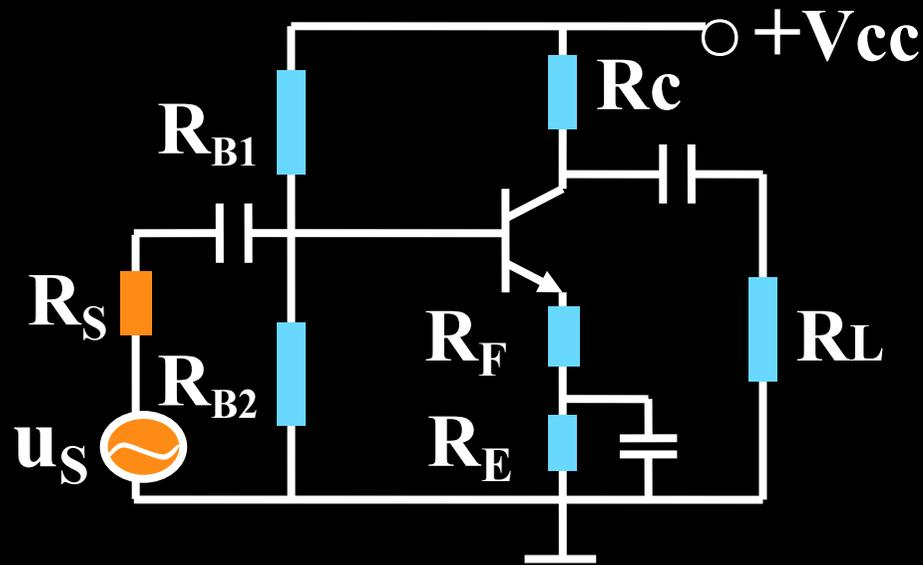
$$U_B = \frac{R_{B2}}{R_{B1} + R_{B2}} \cdot V_{CC}$$
