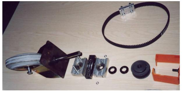
Fig 13: Explosion picture of one steering link
