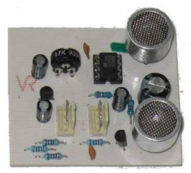
Fig 20: Ultrasonic sensor electronics (final design)
