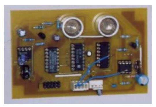
Fig 18: design of a ultra sonic distance sensor with 8-bit bus connector (original design)
