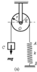
解一：用  $\frac{d}{dt} \left( \frac{\partial T}{\partial \dot{q}_j} \right) - \frac{\partial T}{\partial q_j} = Q_j$  拉氏方程求解。
