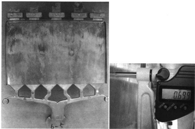
Fig.7 Thin-wall notebook housing with a thickness of 0.7 mm
