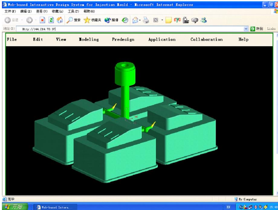
Fig. 7. The cavity layout, the core inserts and the feed system.
