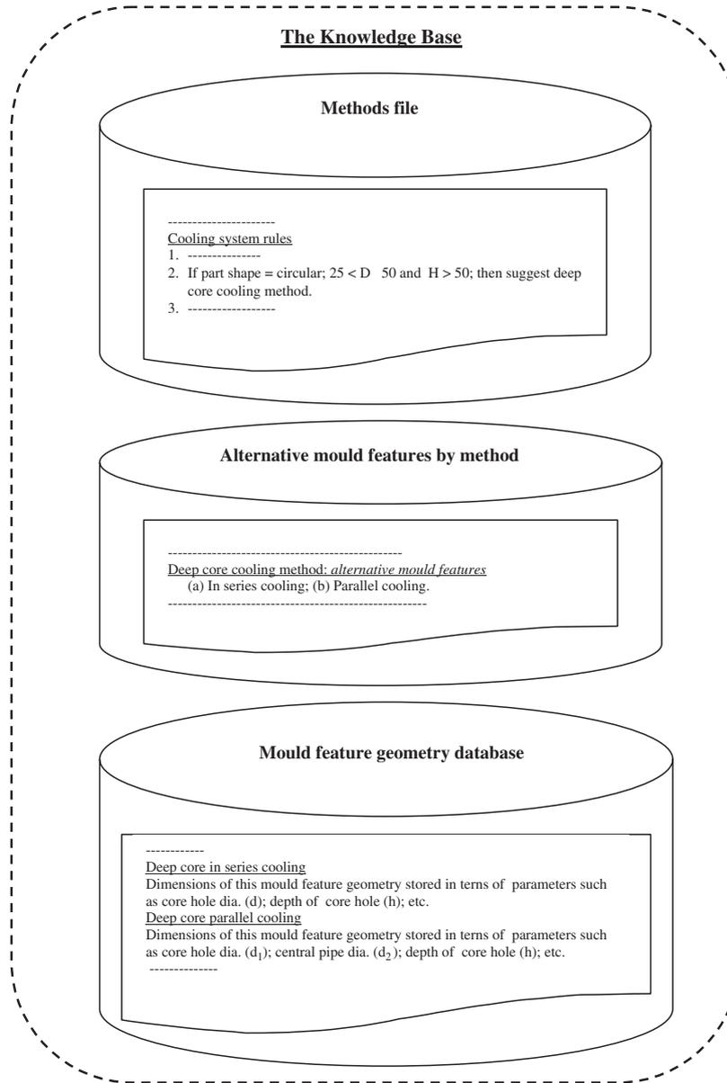
Fig. 5. The schematic representation of the internal structure of the KB.
