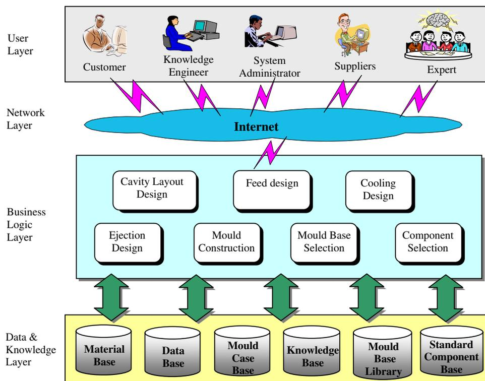
Fig. 2. Architecture of the Internet-based mould design system.
