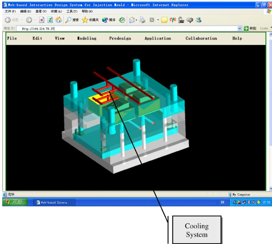
Fig. 9. The detailed design of the cooling system.
