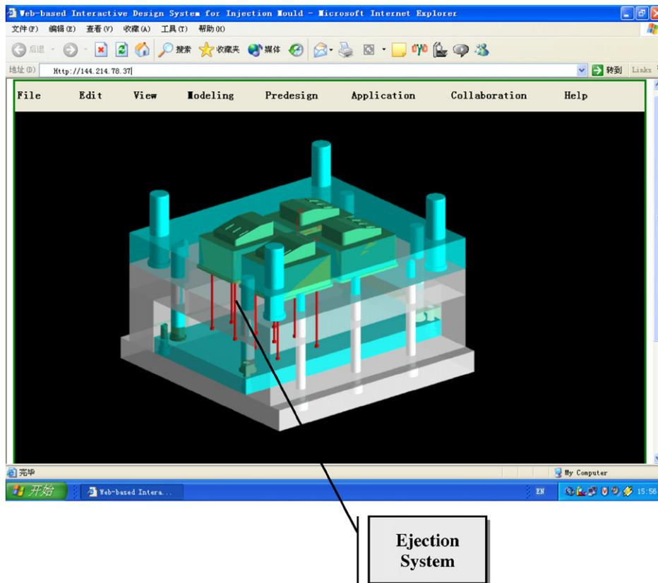
Fig. 10. The detailed design of the ejection system.
