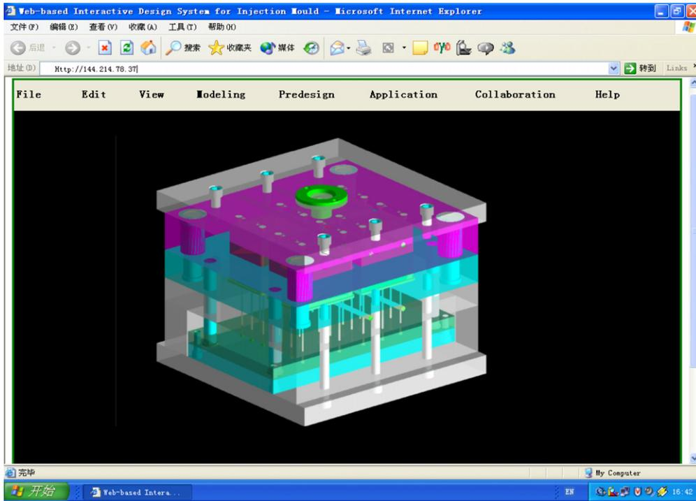
Fig. 11. The finished injection mould for the mouse part.
