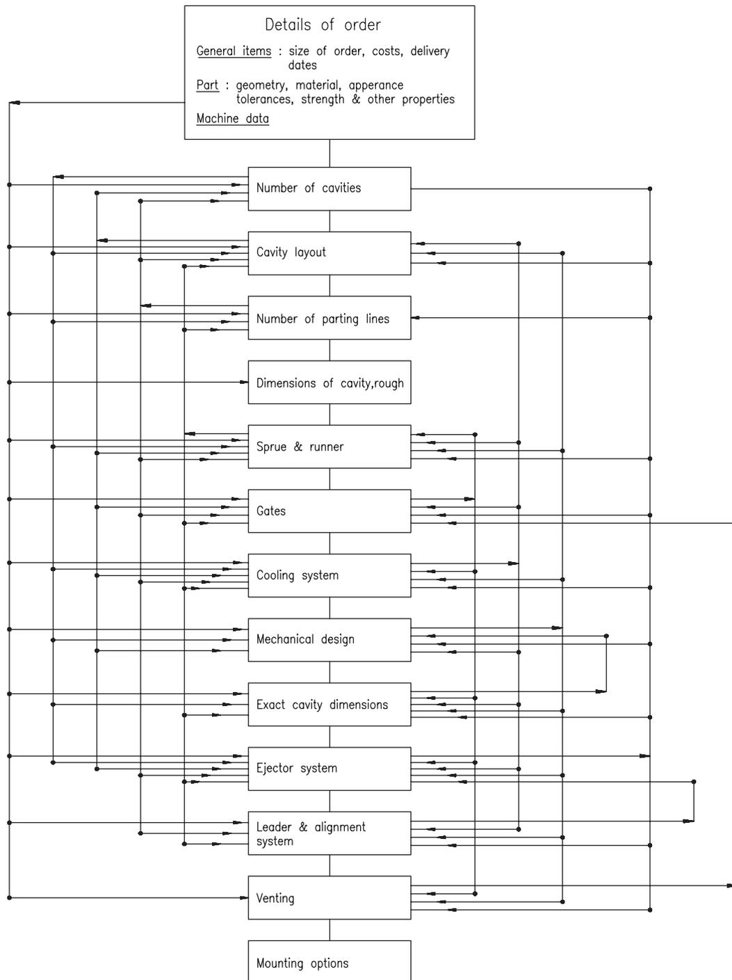
Fig. 1. The general procedure of mould design [1].
