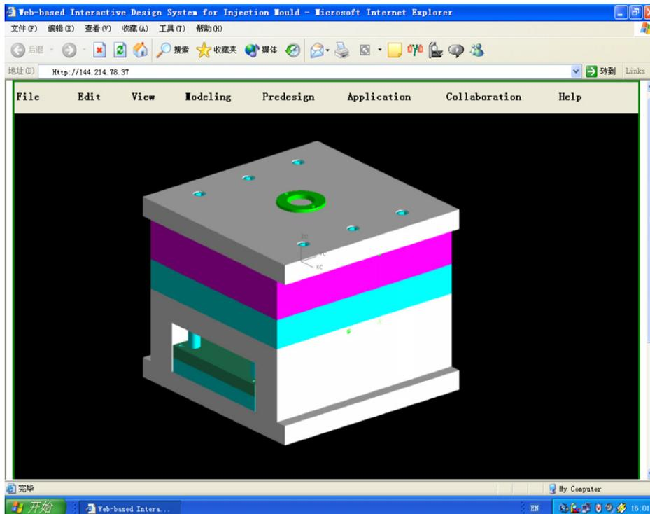
Fig. 8. The detailed design of the mould base.
